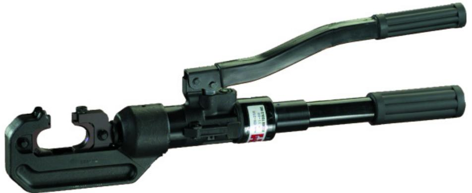
Huskie's **CN-258** is used for service entrance connections up to 4/0, and its bypass cartridge assures all compressions. A two-stage, rapid advance pumping system and threaded collar save compression strokes and time.
