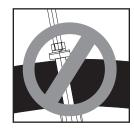
Sagging conduit creates "nodes" which can damage the hanger.
