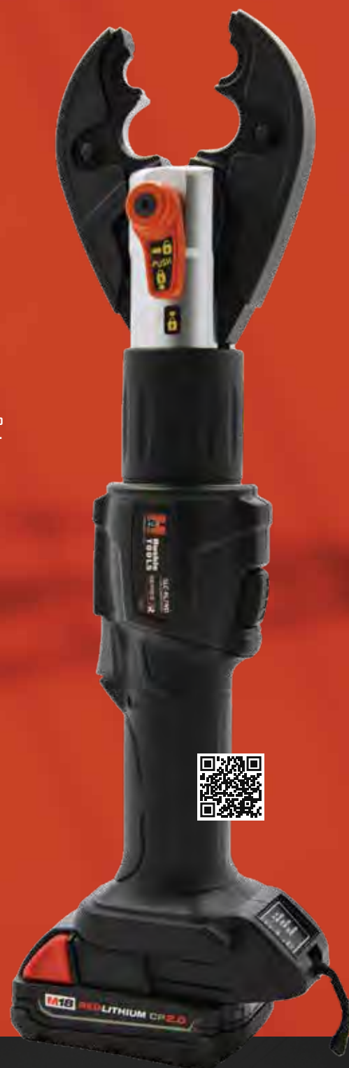
NEW EVS-ACSRJAW Cuts EHS Guy Wire up to 3/8" diameter & copper, aluminum up to 350 MCM, & ACSR up to 556 MCM.
