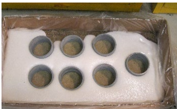
InstaGrout flows and expands after 20 minutes
