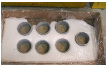
PedFloor flows and expands after 20 minutes
