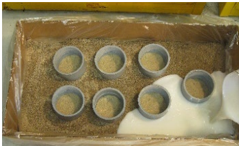
PedFloor is mixed and poured
