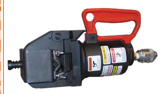
The Huskie **SP-32CC1** is our most durable head unit, its heavy duty design allows it to cut material most other cutter heads will not. It works with most 10,000 psi high pressure pumping systems. Its flip-top latch allows for easy insertion of cutting material. Our unique adjustable heavy duty material clamping system helps to ensure cleaner, safer cutting. The SP-32CC1's cutting blades are easily replaceable. The SP-32CC1 comes with a sturdy metal case.
