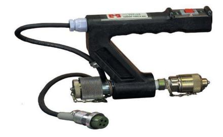
The **URH-14** remote control handle is for use with the R-14EF, R-14EA and REC-P1 pumps. It is equipped with a standard 3/8" high pressure coupler that can be easily matched to your existing tool head. A 10 foot, three wire control cable can be hooked directly to the R-14EF or hard wired to any pump that has similar remote control features. The URH-14 weighs only three pounds and is made of tough, durable, molded plastic with a double insulated on/off switch.
